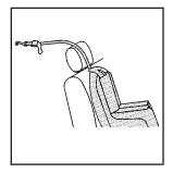
If the position you are using has a fixed head restraint and you are using a single tether, route the tether over the head restraint.
